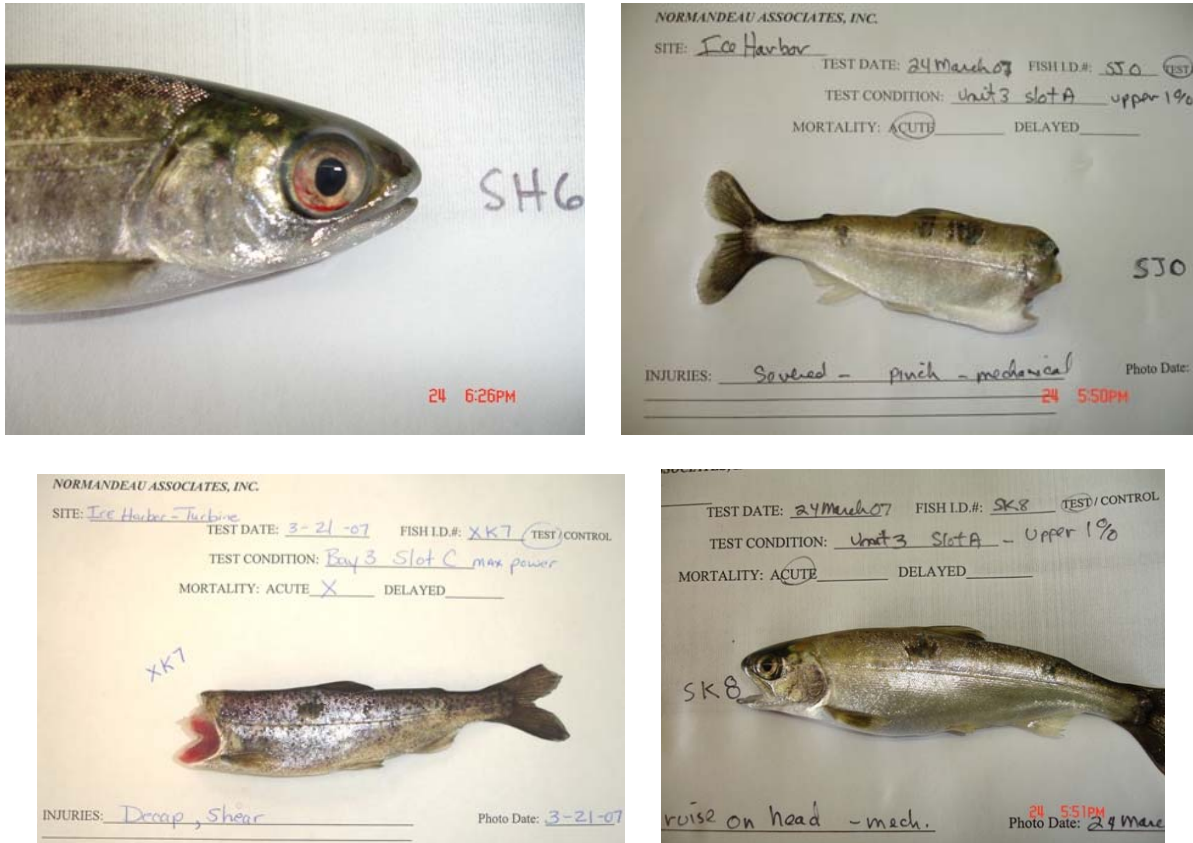
Figure 4-9 Examples of shear injuries (hemorrhaged eye: top left and decapitation forward of the gill arches: bottom left) and mechanical injuries (pinched body: top right and bruise behind head: bottom right) sustained by yearling Chinook salmon passed through turbine Unit 3 at Ice Harbor Dam, March 2007.
